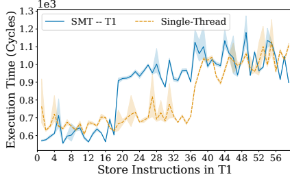
Figure 13: Reverse Engineering the SQ Sharing Mechanism. In single-thread mode, we see a spike in the execution time at 36, exactly the size of our SQ. In SMT mode, T2 only executes NOPs, but still causes T1's SQ to be halved.
